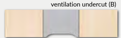
VETRO B - doesn't fulfill ventilation requirements
